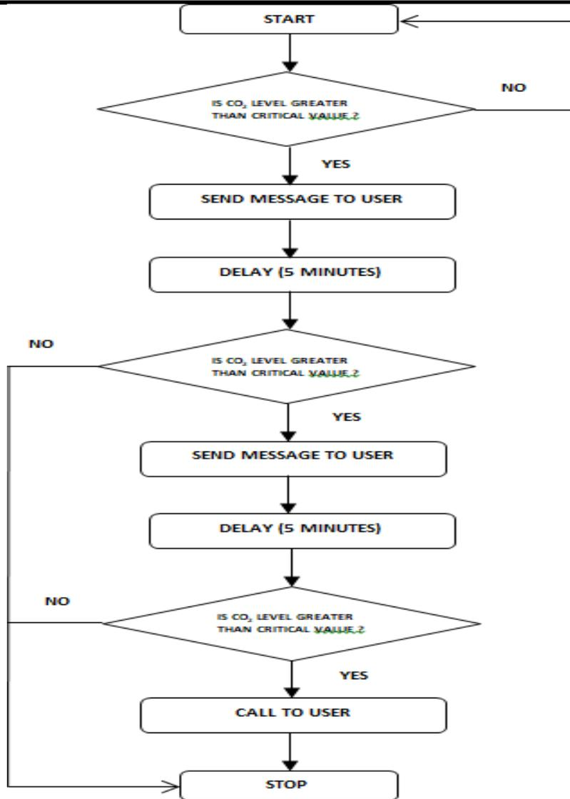
Fig.3 – Flow chart for designed module
