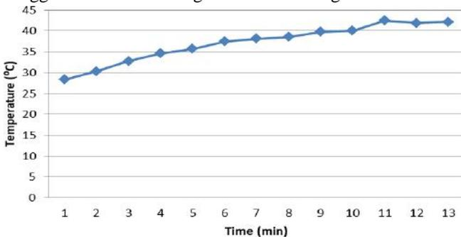
Fig.4 – Analysis of temperature over the time inside the locked car
