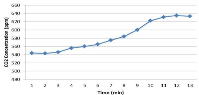
Fig.5– Analysis of CO<sub>2</sub> concentration over the time inside the locked car
