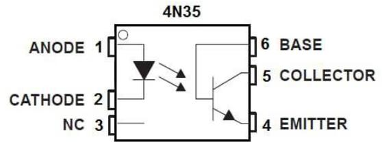
Fig.3. 4N35 Optocoupler pin layout
