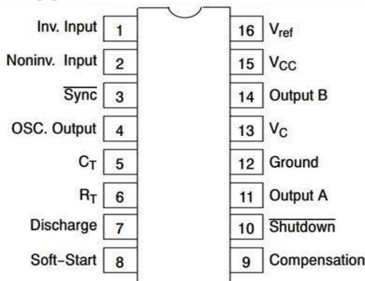
Fig.2. SG3525 pin layout
