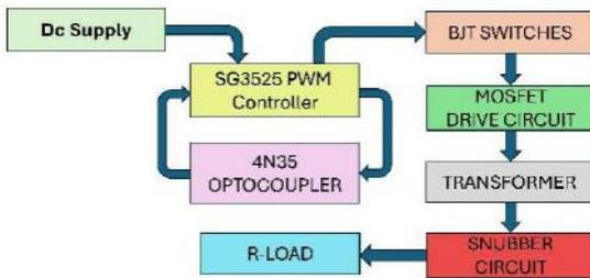
Fig.1. Block diagram of Third Harmonic Less Inverter.
